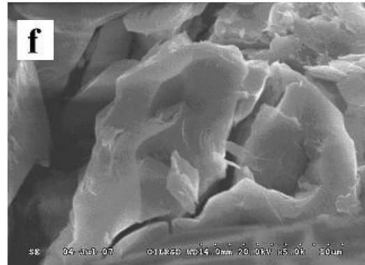
**Figure 2.** SEM photomicrographs of Lakadong reservoir sandstones. *a*, Kaolinite books. *b*, Gypsum crystals. *c*, Intergranular pore. *d*, Glauconite developed in pore space. *e*, Quartz overgrowth. *f*, Microfracture in framework quartz.
