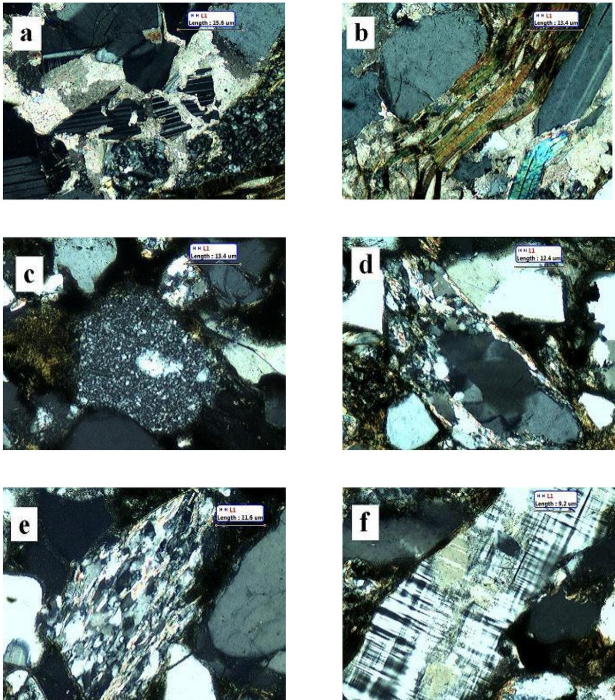
**Figure 3.** Photomicrographs of Lakadong reservoir sandstones. *a*, Dissolution of quartz and feldspar grains (100x). *b*, Dissolution and kink bend of mica flakes (100x). *c*, Authigenic chert (100x). *d*, Rock fragment (100x). *e*, Metamorphic Rock fragment (100x). *f*, Surface corrosion on microcline grains by cementing material (100x).
