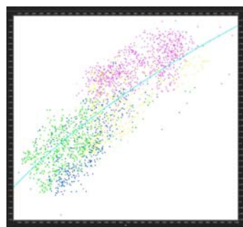
Fig. 7 Cross Plot Vp vs Density colored with well Gardner Law: \rho_{ob}=0.31 \cdot Vp^{0.253}
