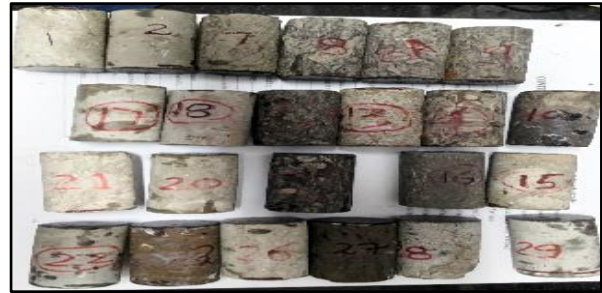
Fig-6 Studied Core plugs samples for acoustics laboratory measurements
