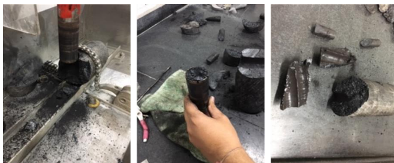
Figure 3: Coal sample breaking during sample preparation
