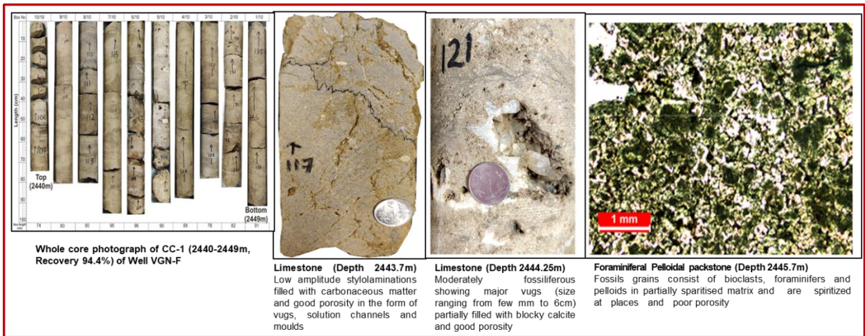
Fig.14: Core analysis (CC#1) belonging to Mid. Eocene carbonate (2440-2449m) of well VGN-F
