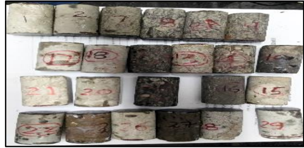
Fig-5 Core plugs samples prepared for acoustics laboratory measurements
