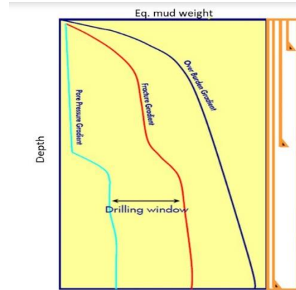
Fig. 3: Plot showing relationship between pore pressure gradient, Fracture gradient and over burden gradient.
