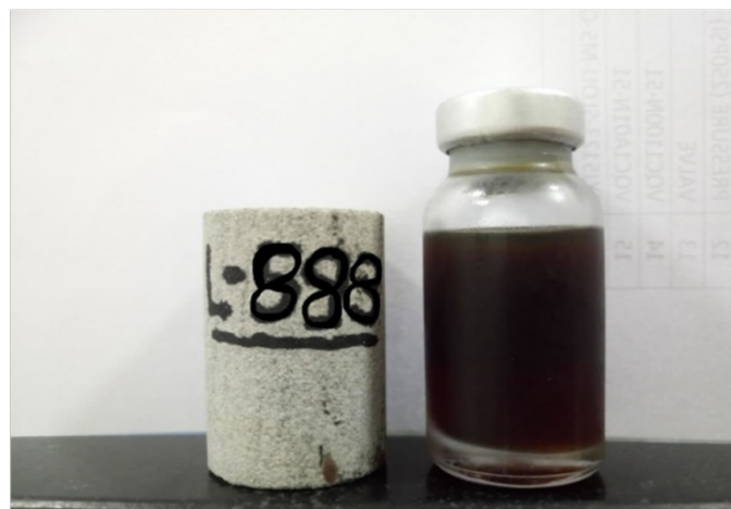
Fig-3B: Oil sample extracted from core
