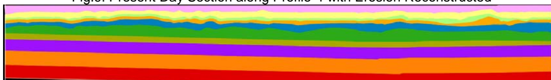
Fig. 10: Sequential Restoration Along Profile - 4 : Anticlines are Restored.
