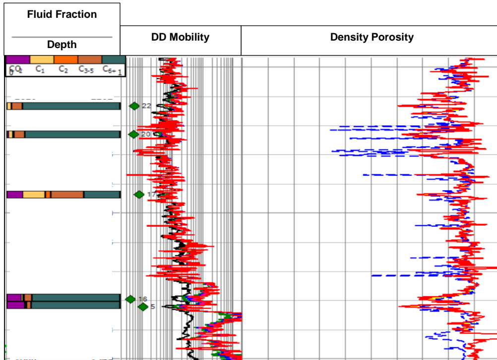
Fig6: Well A: Flow established in basal clastic layer in less than 0.1mD/cP mobility. Presence of moveable oil by Insitu fluid analyzer confirmed reserves within basal clastics. Green fraction represents absorption on the hydrocarbon channel, and blue fraction indicates water based mud filtrate.
