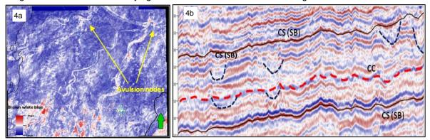
Figure 4: a) Avulsion nodes in northern parts of the area. b) Sequence 2: Dashed red line showing possible correlative unconformity, channels are marked in red.
