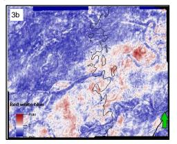
Figure 3: RMS Amplitude slices: a) Straight and meandering channels with feebly developed levees. b) Meandering channels and high amplitude over bank deposits.
