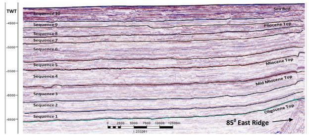
Figure 2: E-W Seismic section showing 10 sequences
