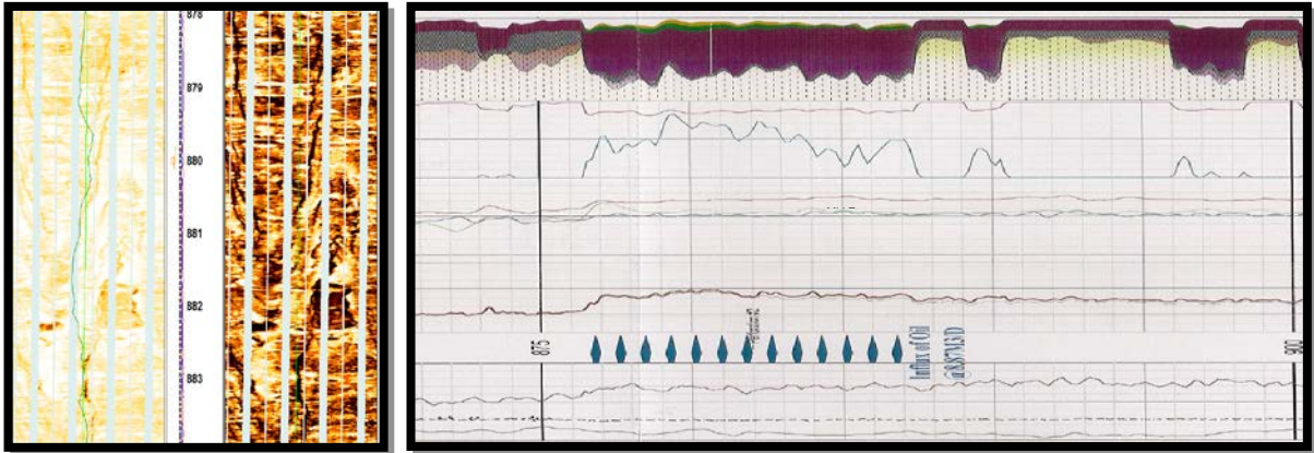
Fig-9: FMI log of Well-D; shows Trapwacke facies with drilling induced fractures indicating maximum horizontal stress direction in NE-SW direction
