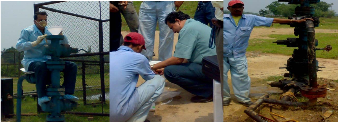
Pic. Injection of tracers in the Geleki Wells
