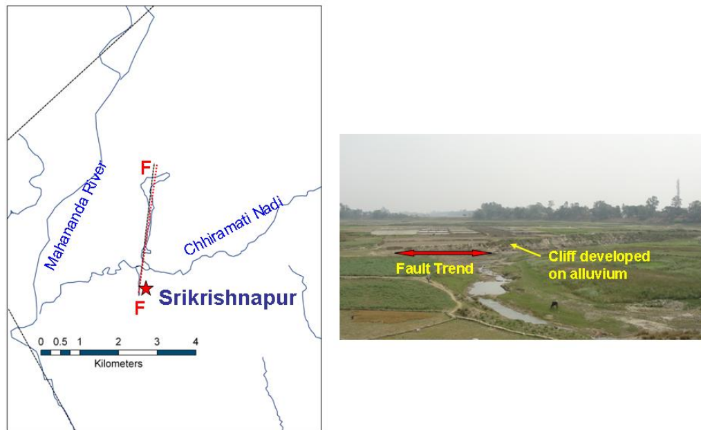
Fig 4. a) Near Srikrishnapur , fault plane of fault FF exposed in alluvium leading to the development of drainage along the fault trace. b) At Mahendra , due to effect of fault FF, pond developed on the downthrown side and prominent incision developed on the unthrown side. Fault plane exposed in alluvium
