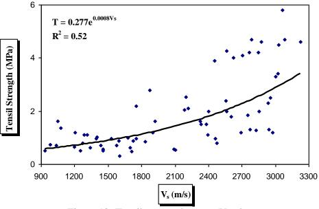
Figure 12: Tensile strength versus V<sub>s</sub> plot
