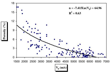
Figure 6: Logarithmic correlation between porosity and V<sub>p</sub>
