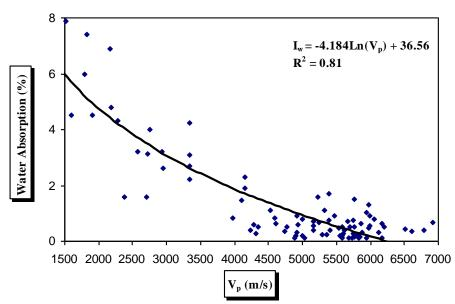
Figure 4: Logarithmic correlation between water absorption and V<sub>p</sub>
