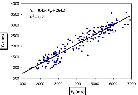
Figure 1: V<sub>s</sub> versus V<sub>p</sub> plot showing a linear relationship
