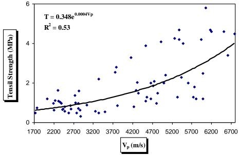
Figure 11: Tensile strength versus V<sub>p</sub> plot
