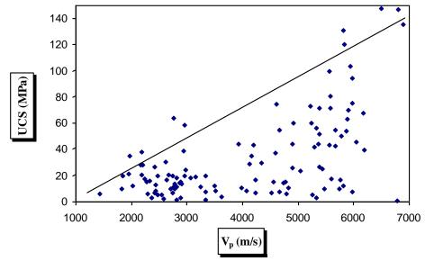
Figure 8: Uniaxial compressive strength versus V<sub>p</sub>
